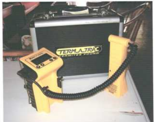
TermaTrak unit, borrowed from Protec Corporation, as a device to detect and locate active termite infestations (positioned here on top of an infestation in a bookshelf in the living room, main house, Guana Island).
